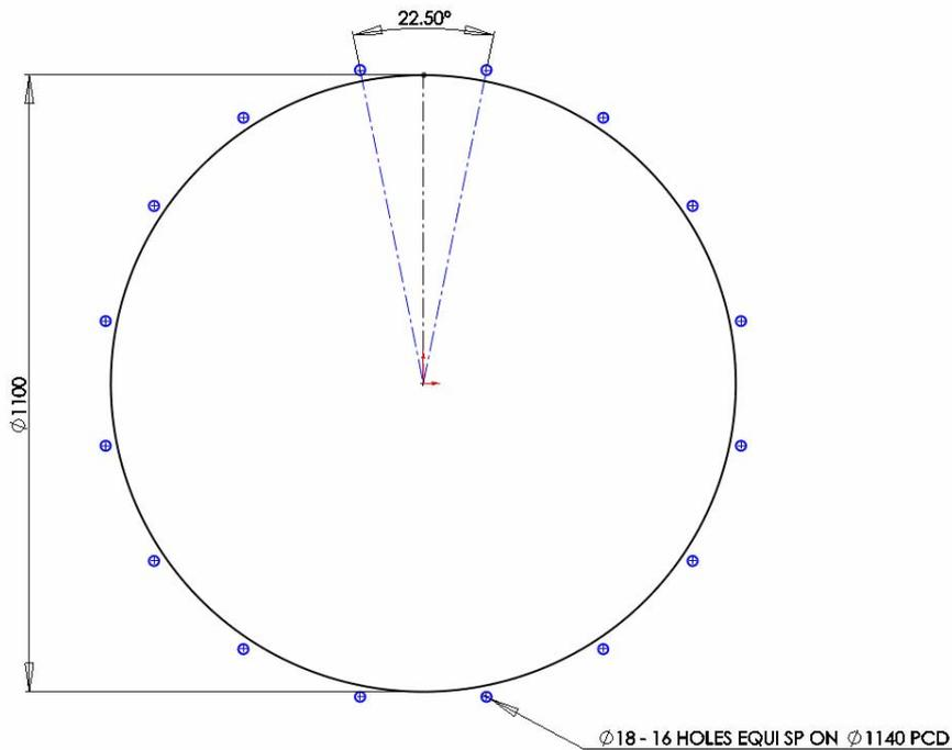
**Figure 5: Weapon Ring Fixing Footprint**
