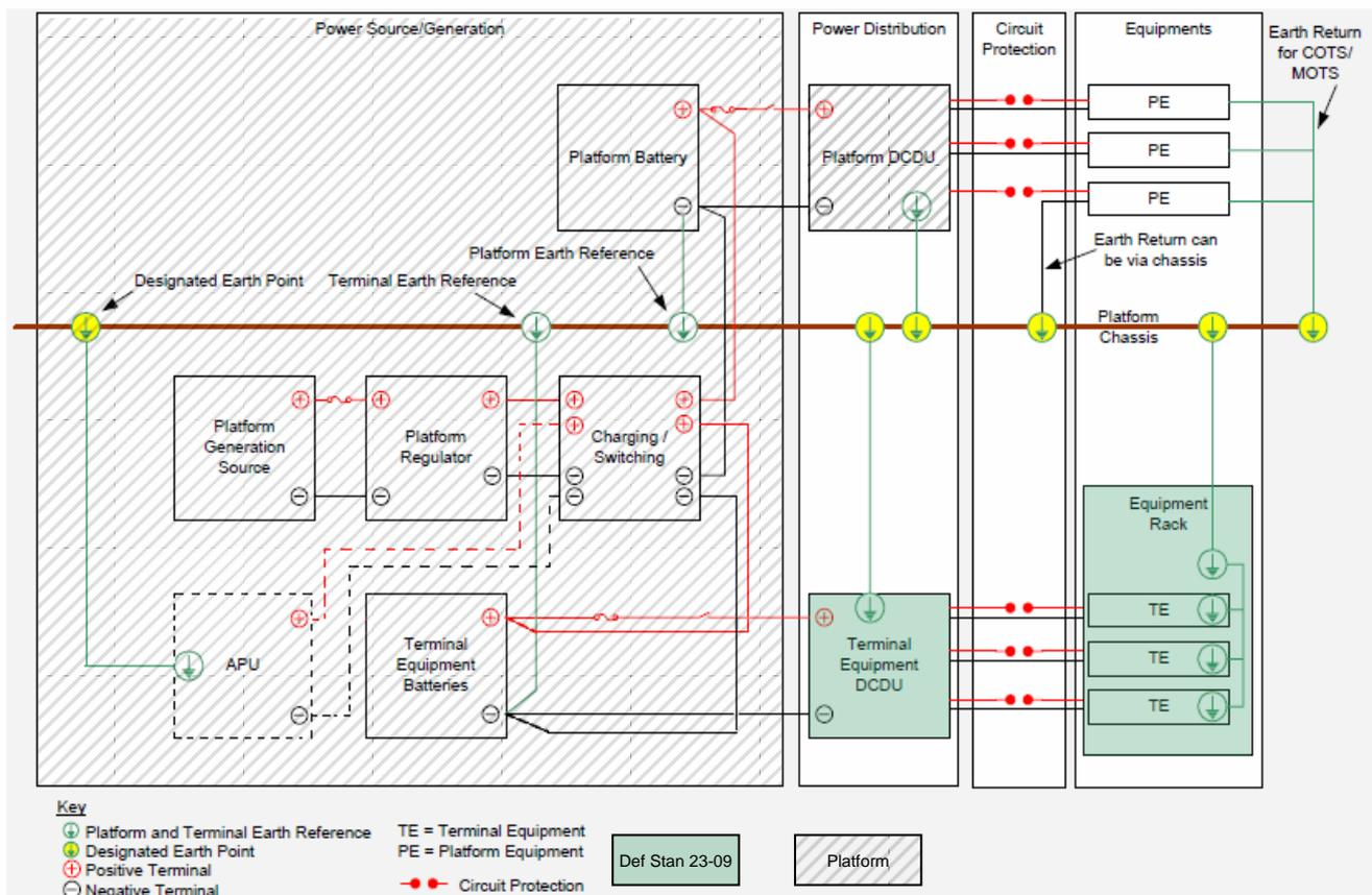
Figure 3: Example Power System Architecture
